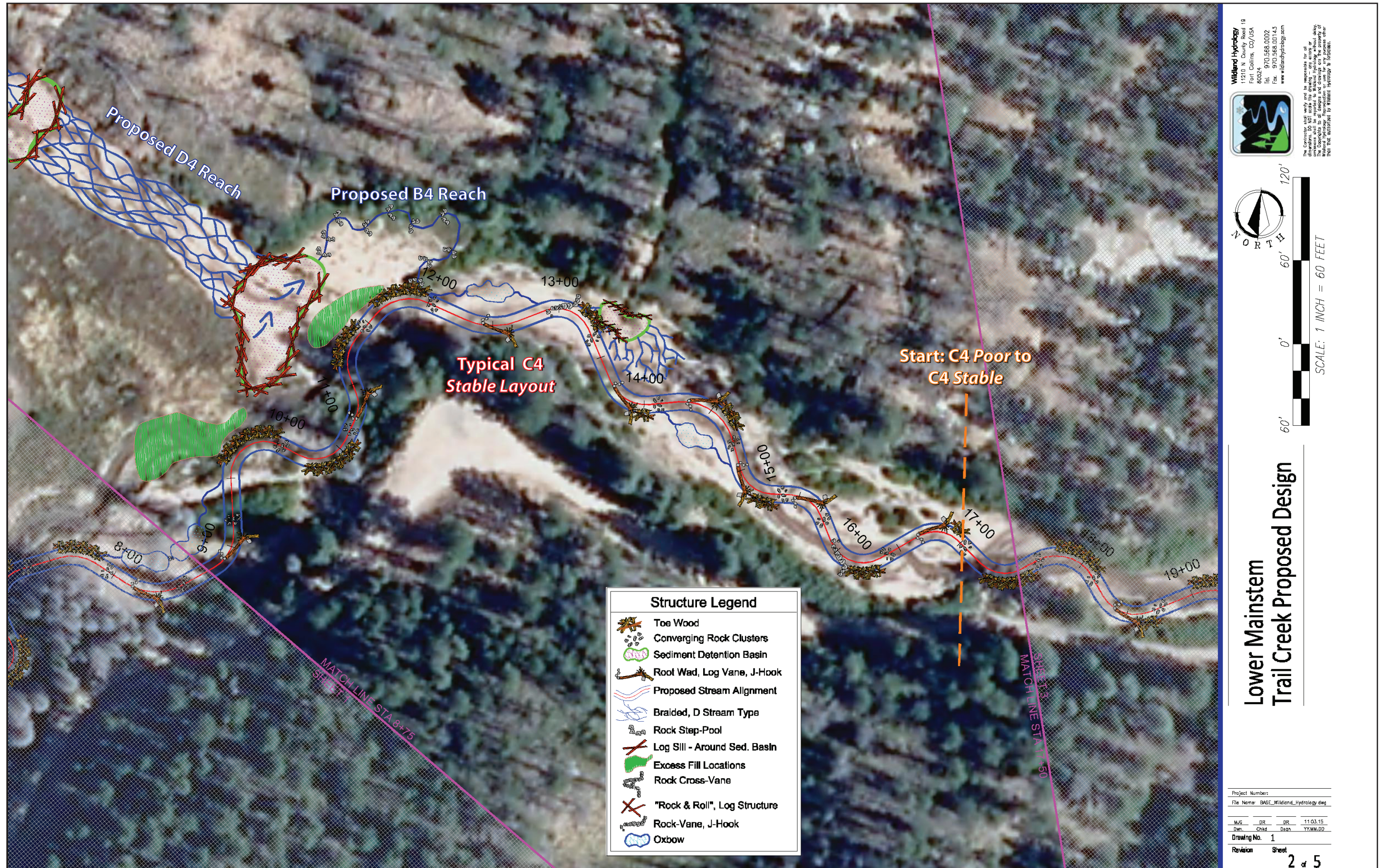
Figure 42. The general proposed design for lower Trail Creek for the area depicted in Sheet 2 in Figure 40.
