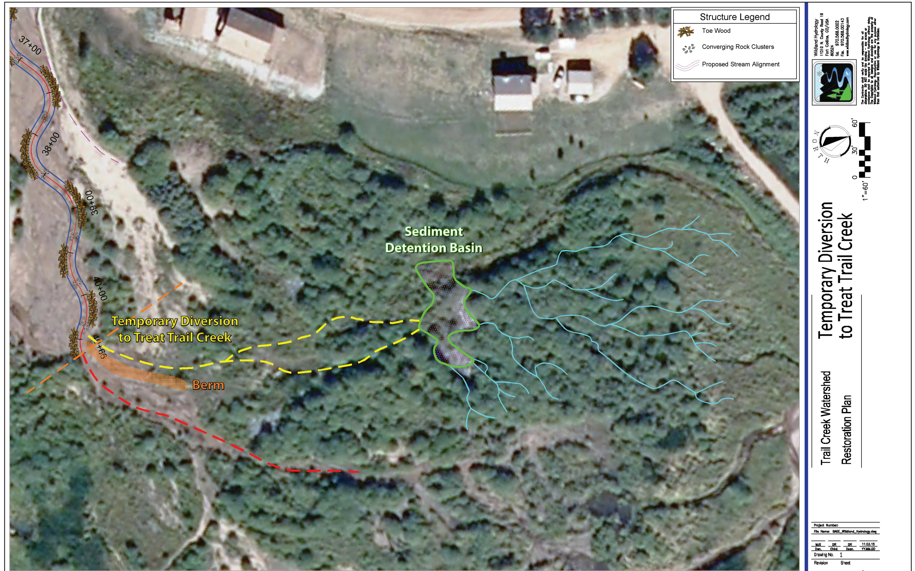
Figure 46. The proposed location of a flow diversion for water quality control during construction using the riparian area for natural filtration and sediment detention.
