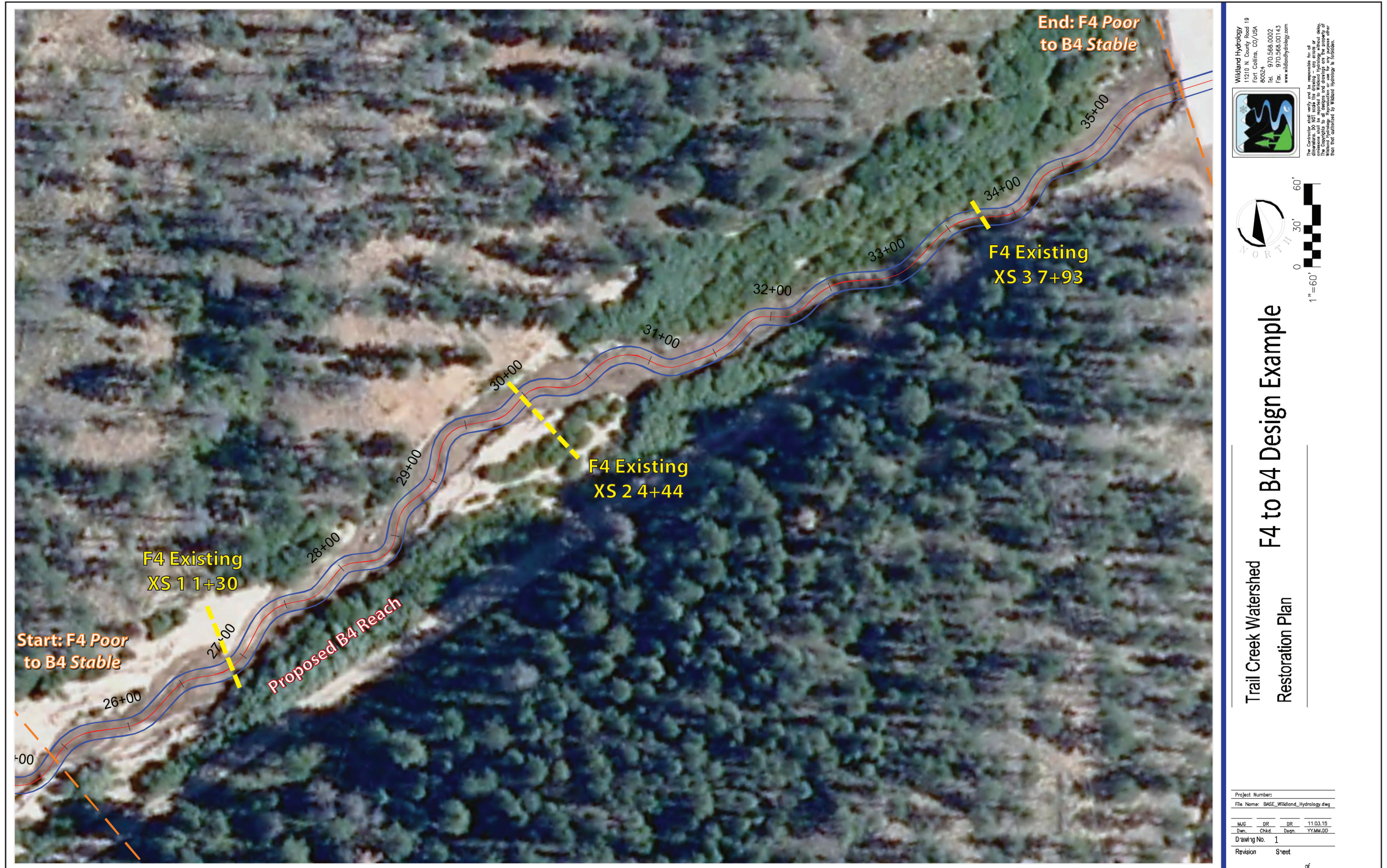
Figure 62. Plan view of the proposed conversion of the F4 to B4 stream type from the West Creek road upstream 1,000 ft to proposed station 25+40, including the existing F4 cross-section locations.
