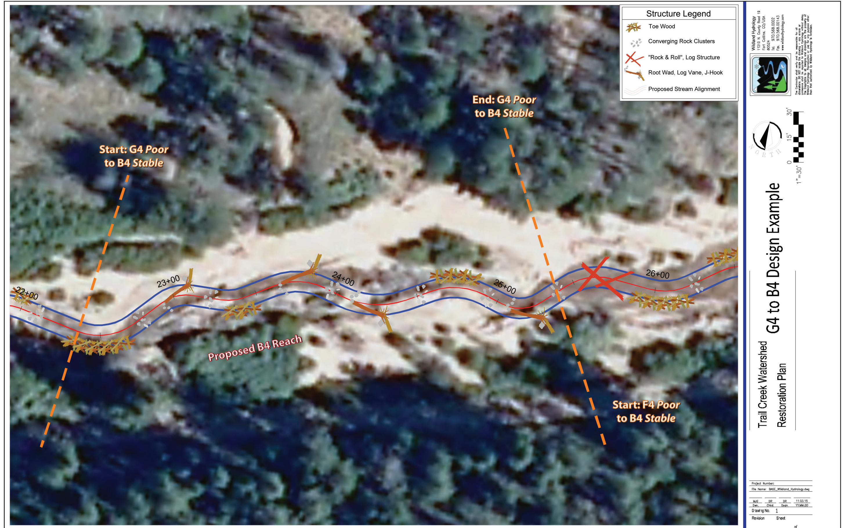
Figure 80. The proposed plan view layout of the G4 to B4 conversion depicting the stabilization and fish enhancement structures.
