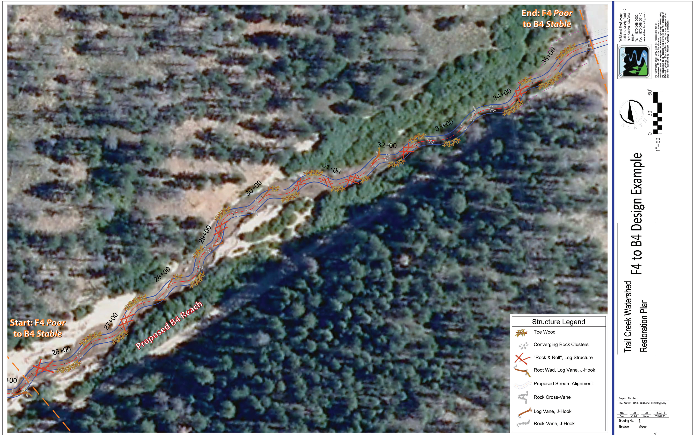
Figure 68. The proposed plan view layout of the F4 to B4 conversion depicting the stabilization and fish enhancement structures.
