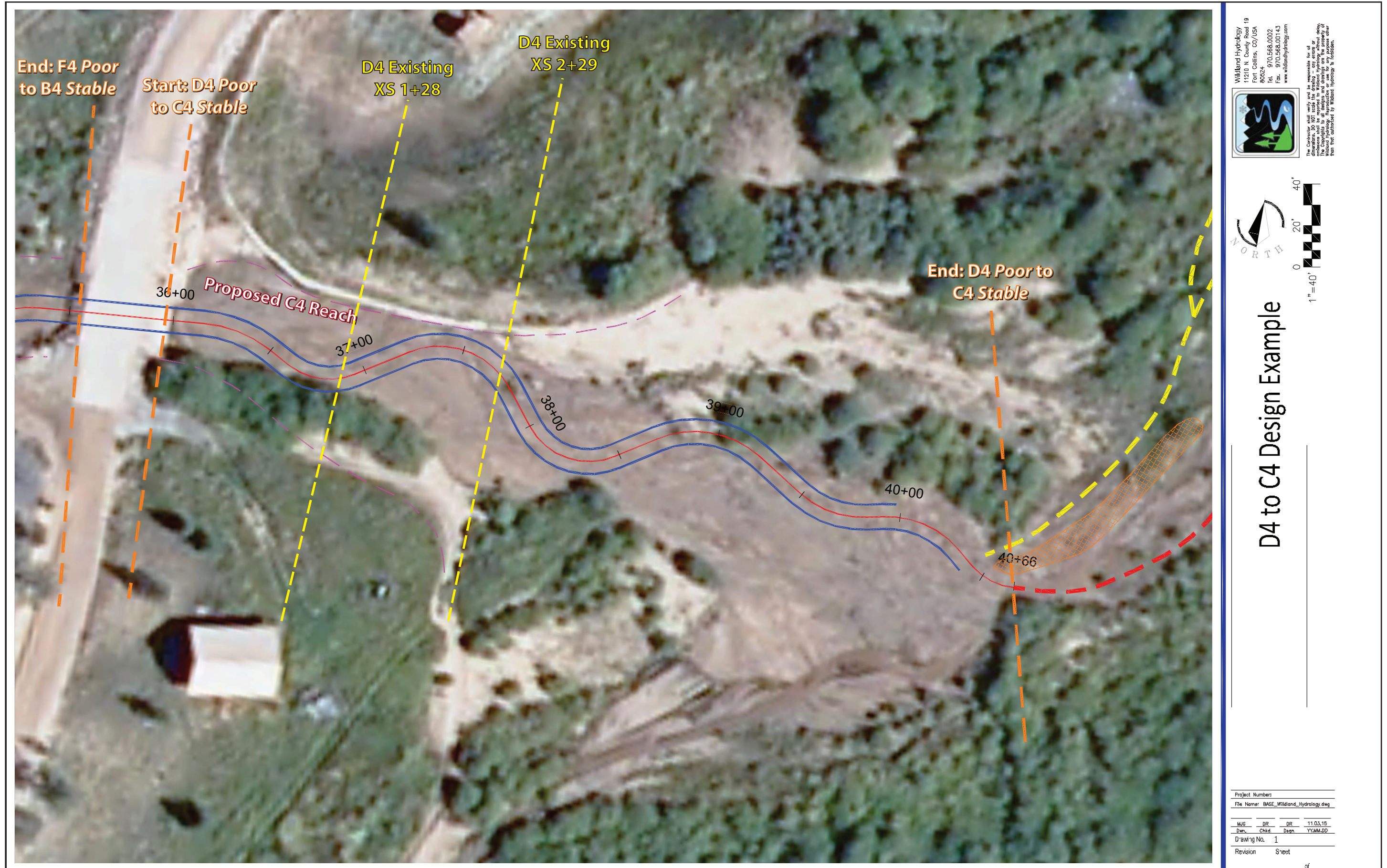
Figure 48. Plan view of the alignment for the proposed C4 stream type, including the existing cross-section locations of the D4 stream type.
