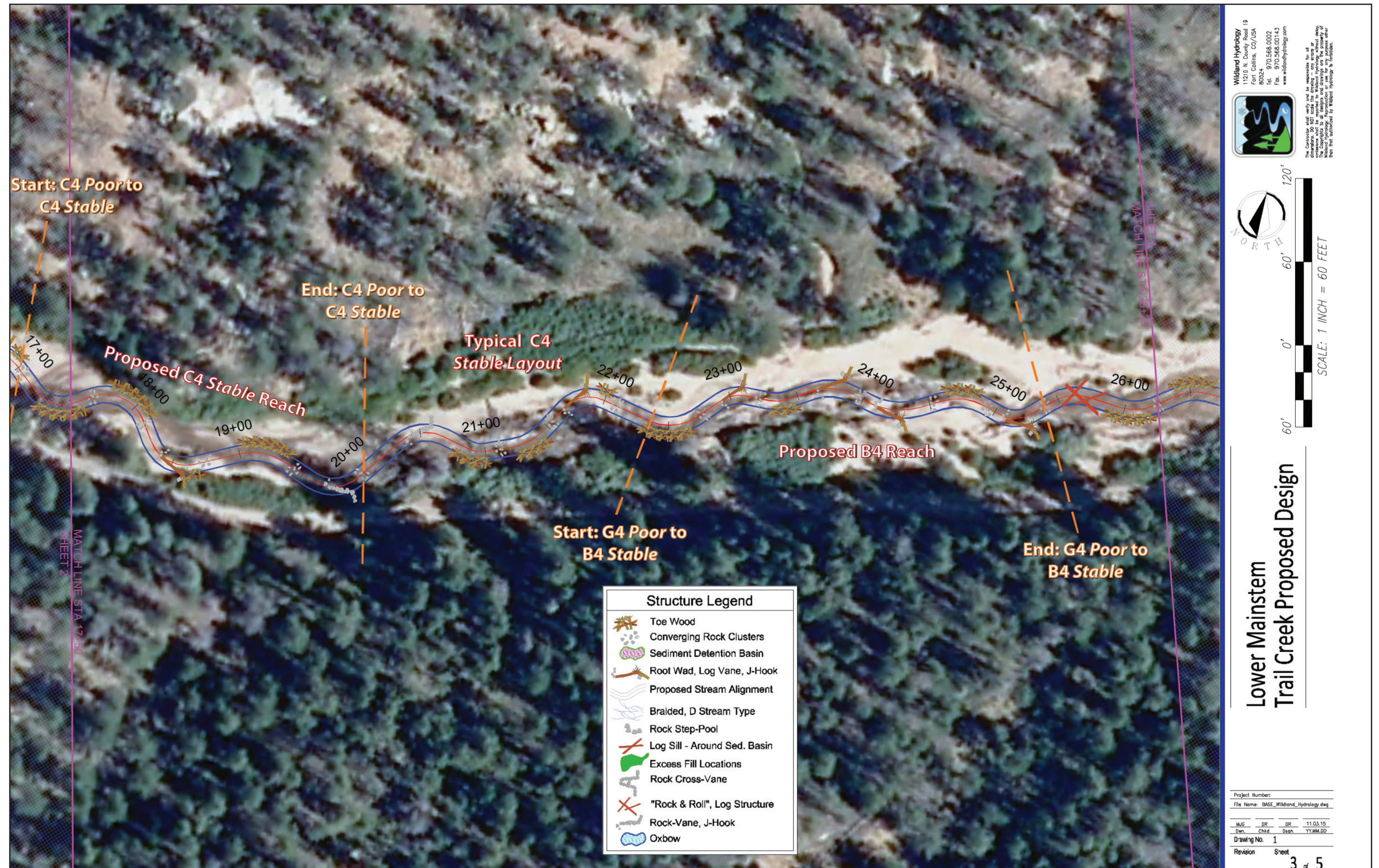
Figure 43. The general proposed design for lower Trail Creek for the area depicted in Sheet 3 in Figure 40.
