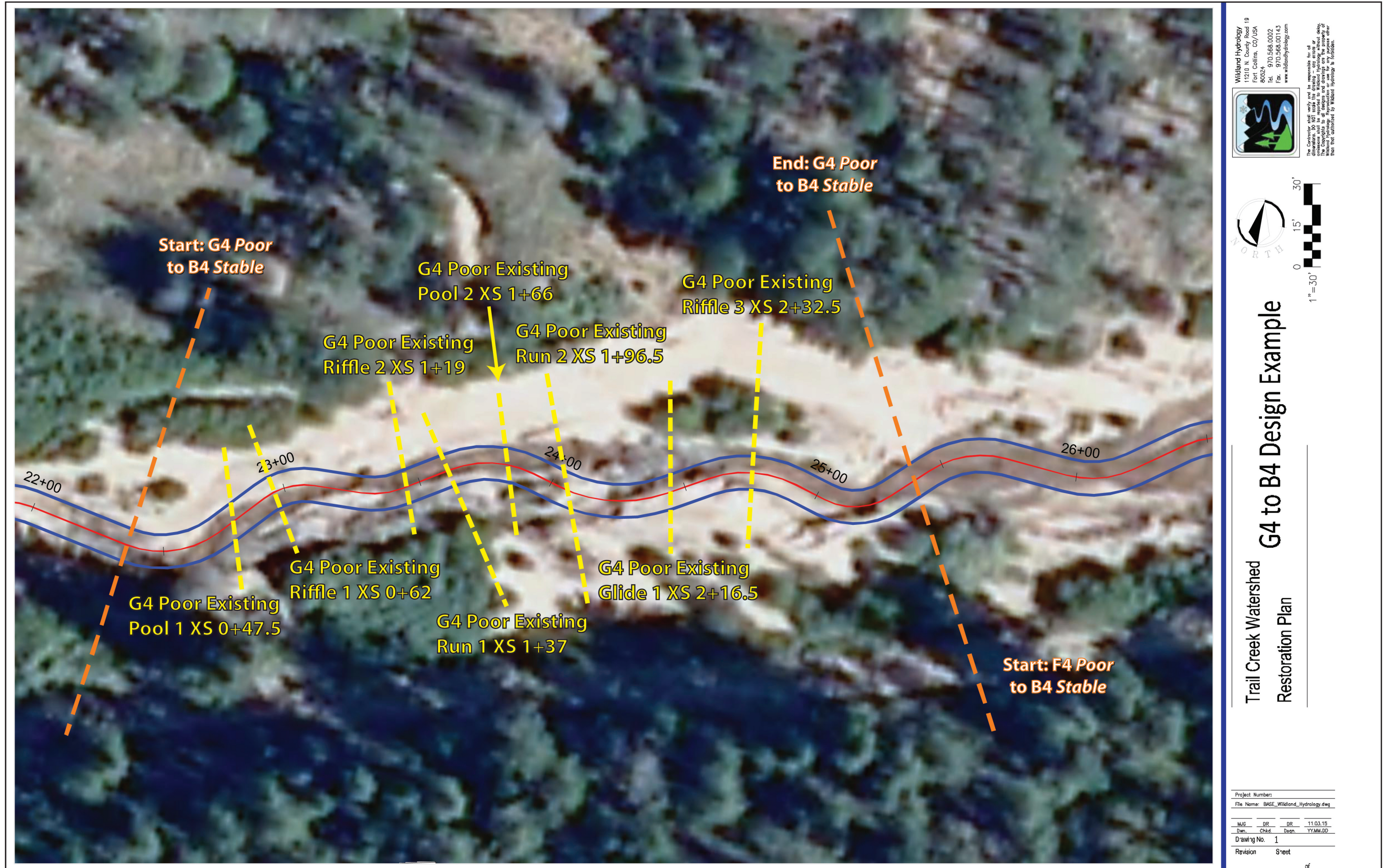
Figure 70. Plan view of the proposed conversion of the G4 to B4 stream type, including the existing G4 cross-section locations.
