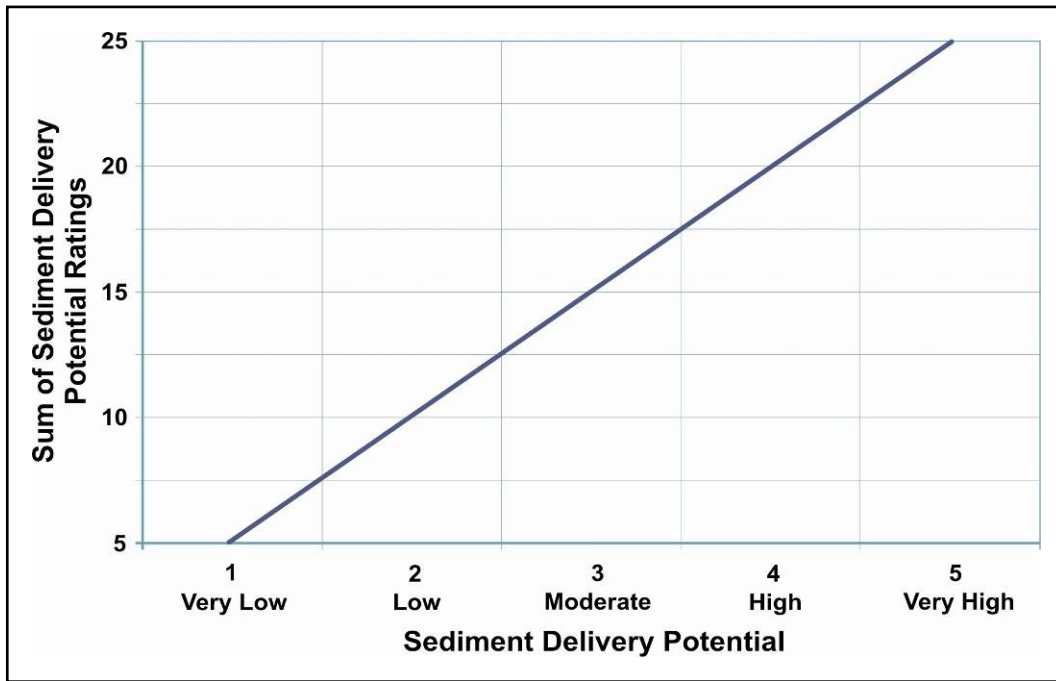
Figure 4-13. Overall sediment delivery risk based on the sum of individual sediment delivery risk ratings.
