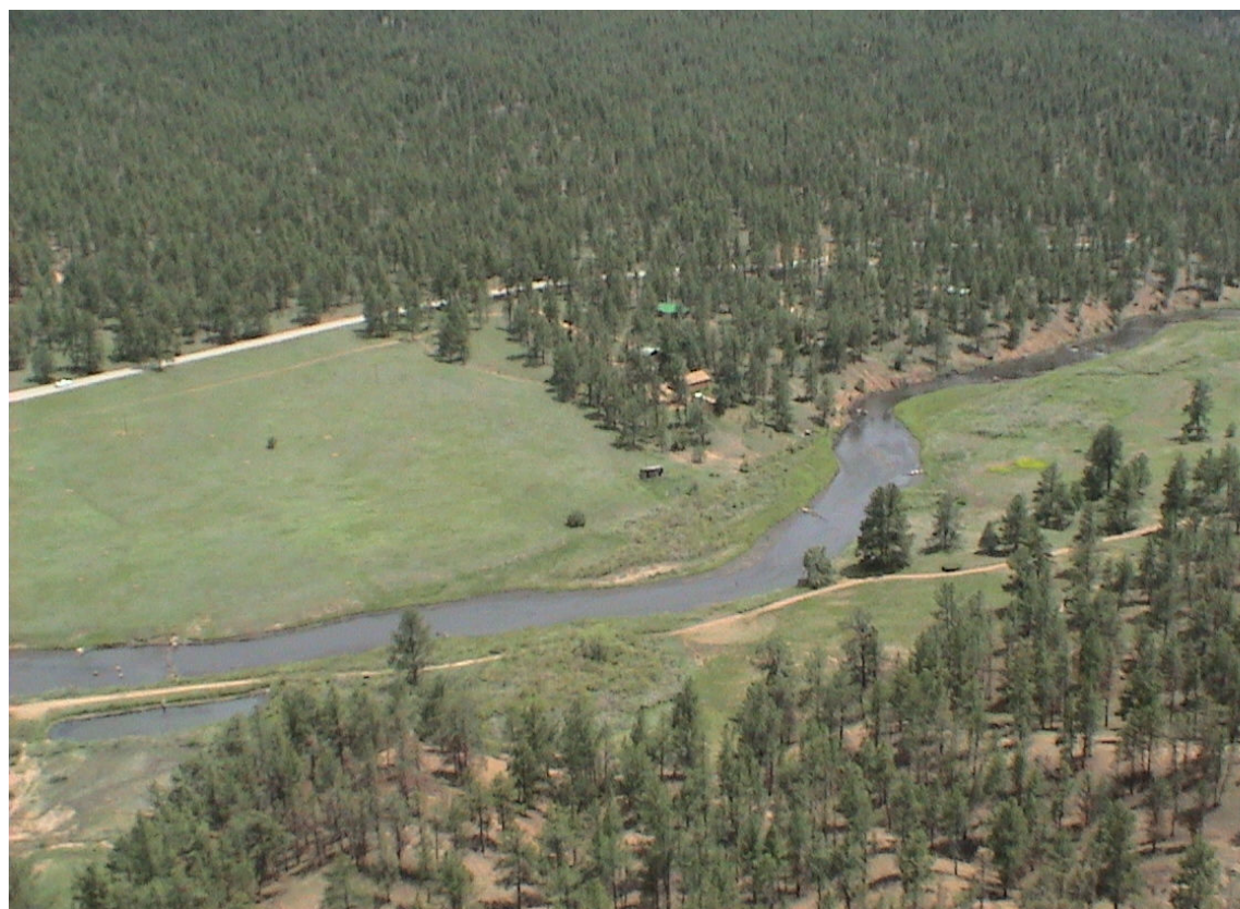
River over-widening due to miss-aligned boulder vanes. Swayback Ranch, CO
