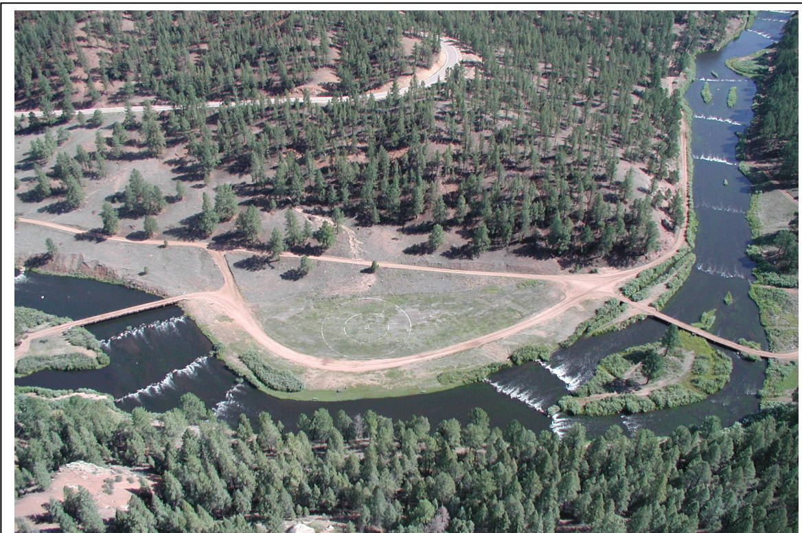
Example of river over-widening due to poorly configured drop structures. Wigwam Club, CO
